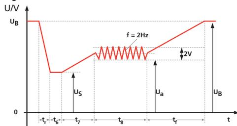
**Voltage transient at engine start-up**
